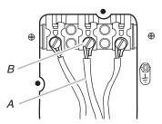
A. Neutral wire (white or center wire) B. Center terminal block screw
